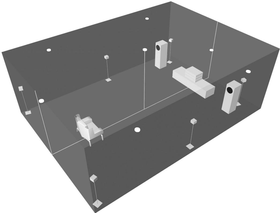
For the use in recording studios please use the same setup, but mount the Hpro a little higher on microphone stands or wall brackets.
