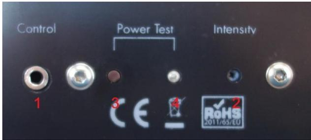
To check whether the batteries are OK, press the button (3).
